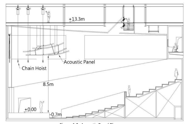
Figure 1.2- Acoustic Panel Plan
