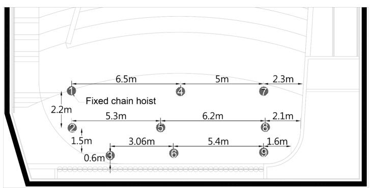
Figure 1.4 - Stage Hoisting plan
