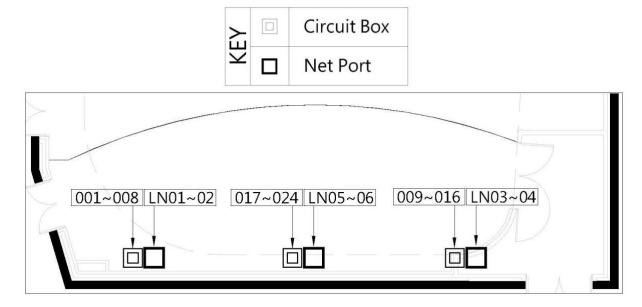
Figure 2.3.1- Stage Area Lighting Circuit Layout
