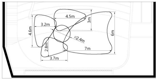
Figure 1.3- Acoustic Panel Plan
