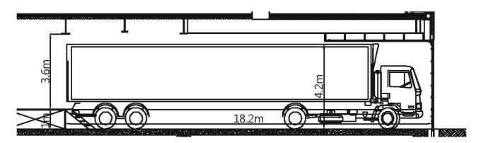
Figure 4.2- East Loading Dock Section
