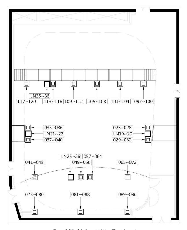
Figure 2.3.2- Grid Area-Lighting Circuit Layout
